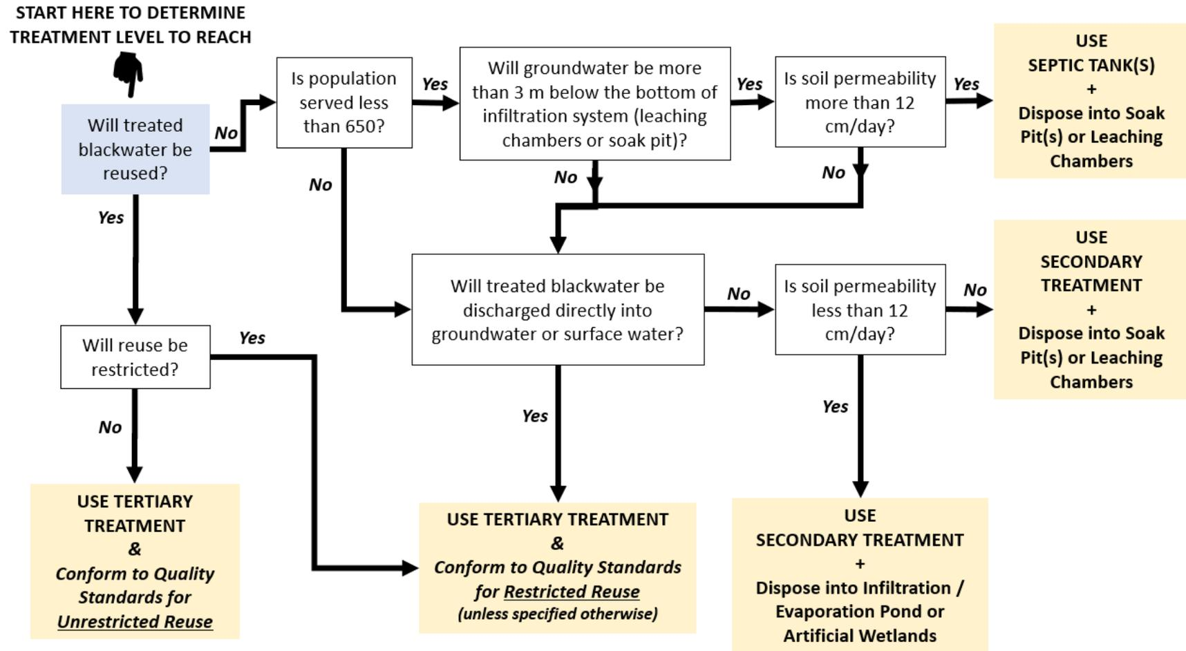
\*Sub-surface infiltration from soak-pit(s) or leaching chambers is to be considered as groundwater recharge when a 3 meters distance between the bottom of the infiltration system and the groundwater table cannot be respected
