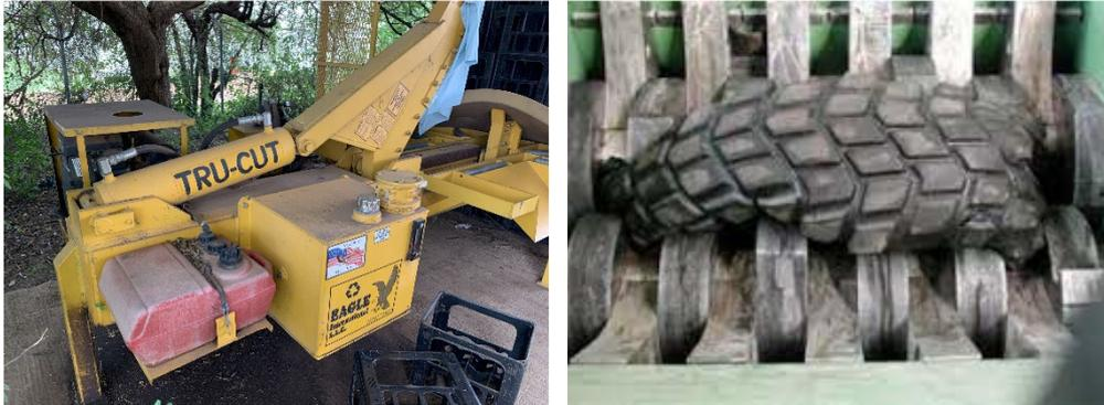
**Figure 51: Tyre cutter and shredding tyres**
