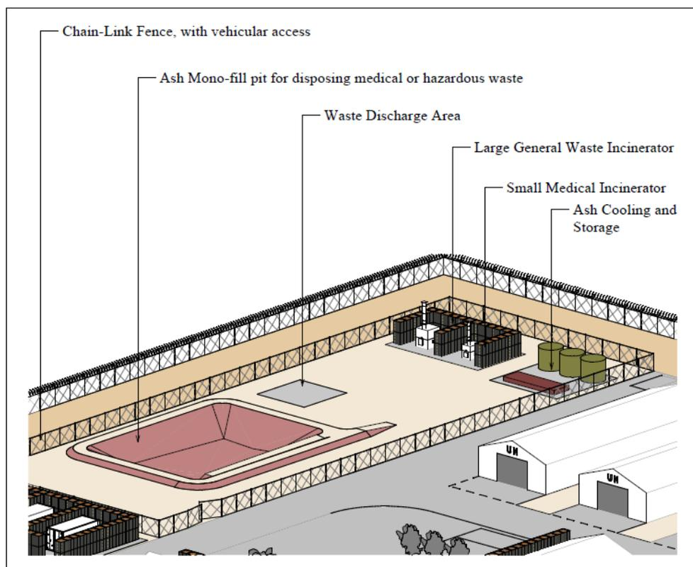
**Figure 5: WMY showing incineration area and ash mono-fill**
