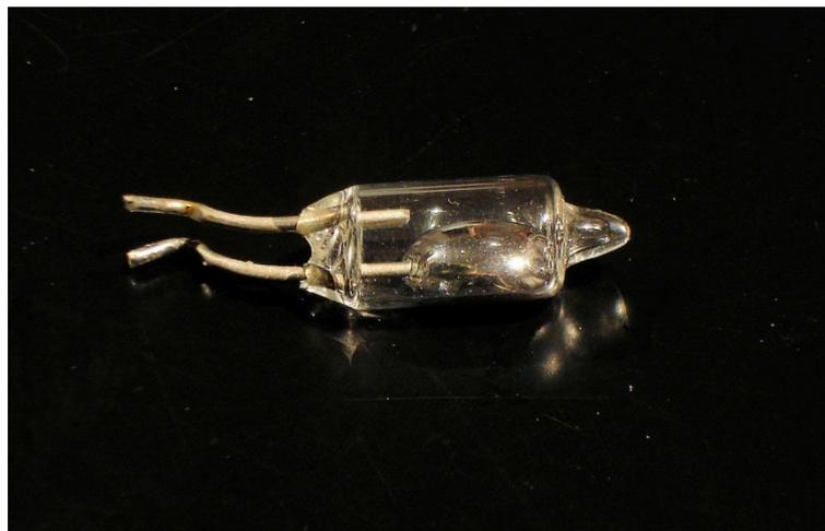
**Figure 69: Mercury switch showing bead of mercury**
