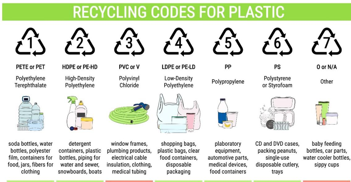
**Figure 9: Universal plastic coding system**
