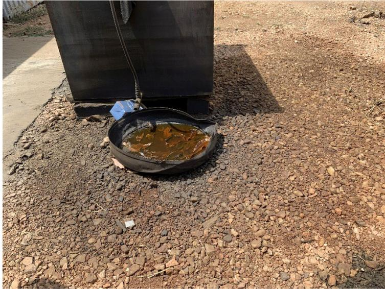
**Figure 63: Examples of poor management of POL products**
