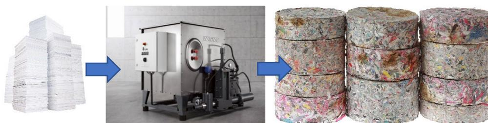
**Figure 16: An automated briquette machine and produced briquettes**
