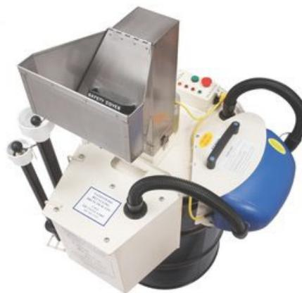
**Figure 41: Fluorescent bulb crusher**
