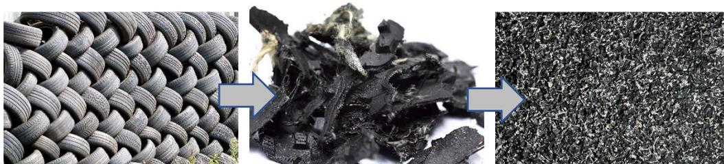
**Figure 52: Waste tyres shredded and processed to granules**
