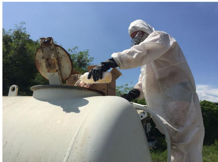
Figure 72: Alkaline hydrolysis treatment for waste pesticides
