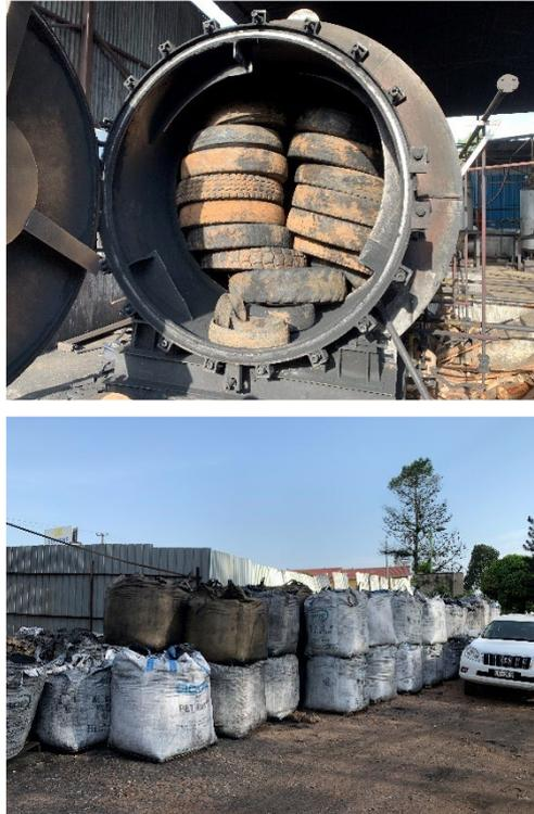
**Figure 53: Pyrolysis of waste tyres for oil extraction and carbonized wastes sold for fuel to a cement kiln**
