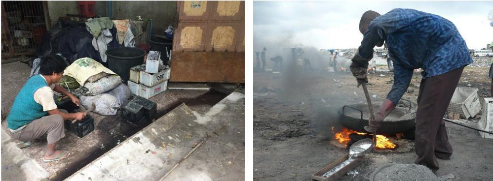
**Figure 33: Inappropriate recycling of lead acid batteries** (source: Oeko-Institut)
