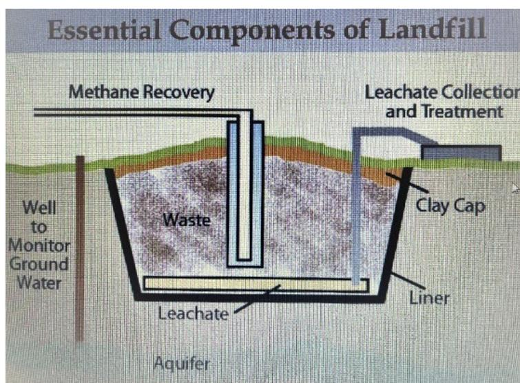
**Figure 22: Schematic for landfill site**
