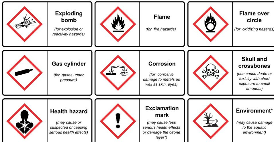
**Figure 26: GHS Hazard Communication Standard Pictograms**
