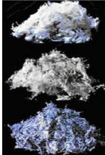
Figure 66: Three main types of asbestos
