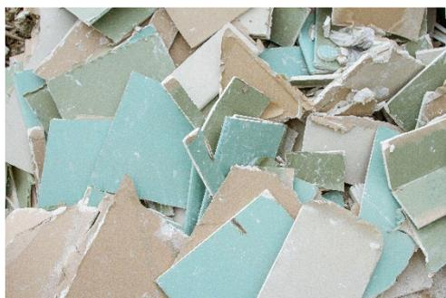
**Figure 20: Drywall plasterboard waste**
